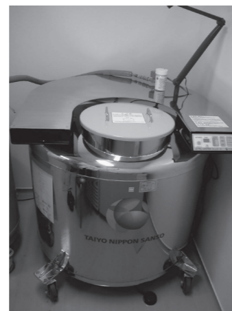
Fig.2 Large liquid nitrogen tank G430-S (Taiyo Nippon Sanso Coporation)
