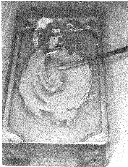
Fig. 10-14. Maximum amount of powder must be incorporated into a given quantity of liquid and still the mass must be plastic enough to allow proper cementation of castings.
