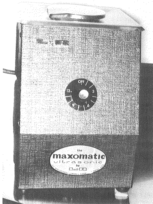
Fig. 10-8. Ultrasonic cleaner unit for cleansing of castings of polishing materials before cementation.
