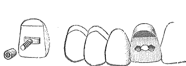
Fig. 851.—Left, Pins Bent and Screw Attached. Right, Backing Slatted and Drilled for Reception of Facing
