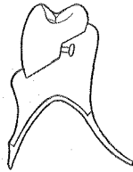
Fig. 72.—Sectional View of Base Showing Finished Shoulders with Vulcanite in Position
