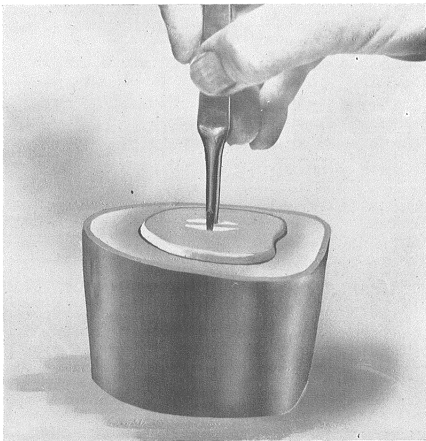
Fig. 48.— Lifting Model from Matrix
