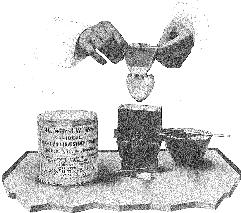
Fig. 86.—Introducing the Partially Invested Wax Model in Flask
