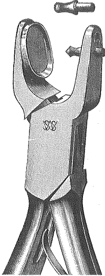
Fig. 854.—Riveting Punch, Showing Cup Beak and Two Riveting Points (Shriver)
