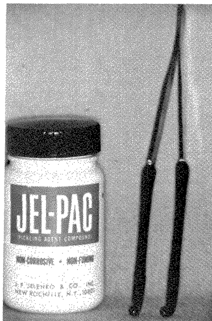
Fig. 8-46. Good pickling solution and Saf-T-Forceps. Contamination is not a problem with these special forceps.
