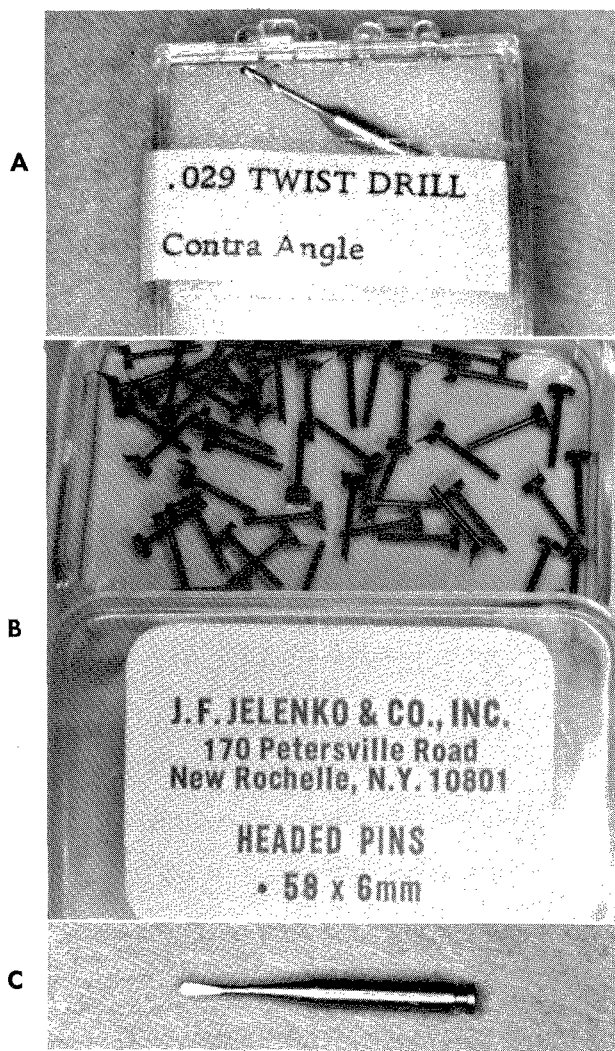
Fig. 6-34. A, Twist drill. B, Sized headed pins (Perlon). C, Bibeveled carbide center drill.
