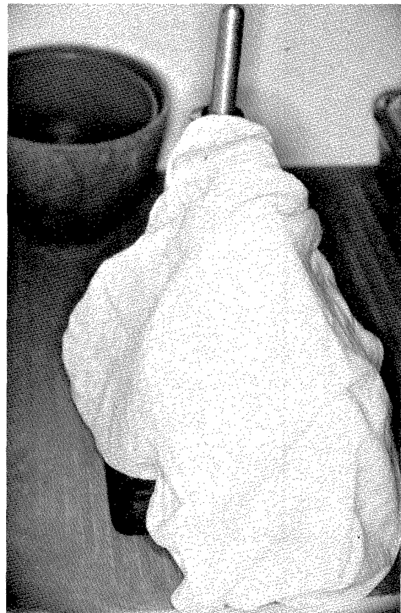
Fig. 7-72. Whole assembly is covered with a wet towel to obtain an atmosphere close to 100% humidity.
