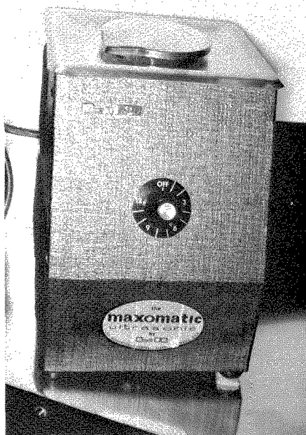
Fig. 8-55. Ultrasonic cleaning unit used for cleansing of castings.
