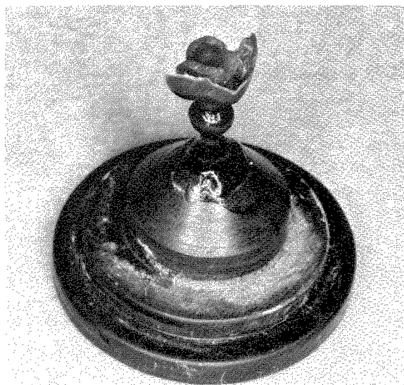
Fig. 8-18. Use of a reservoir helps eliminate porosity.
