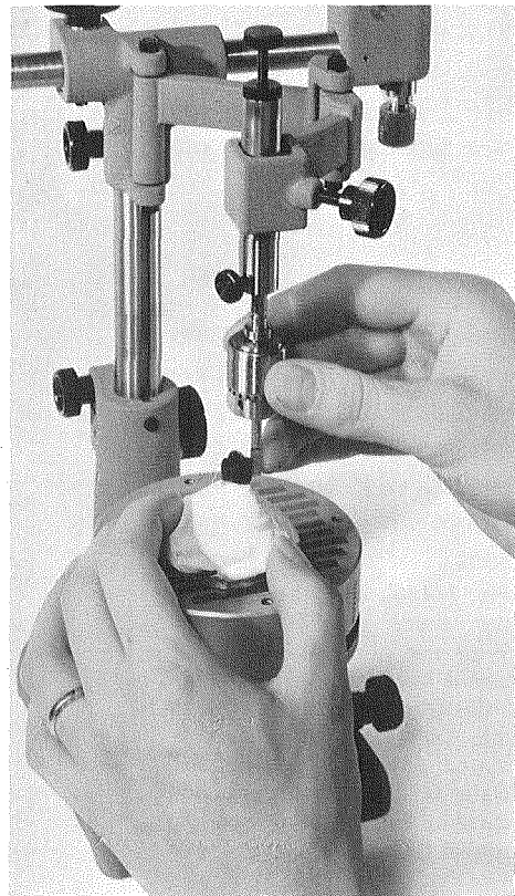
Fig. 113 With wax knives fastened in the large chuck of the parallelometer and through the use of the pantostat as shown here, the walls of the future CSP matrix are trimmed parallel. The best shaving angle must be tried out individually.
