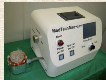
Fig.2: Newly assembled clinical console and motor-driver.
