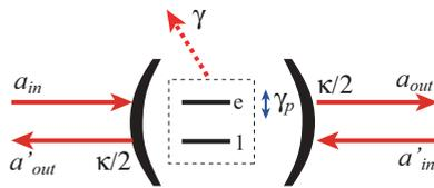
FIG. 2. (Color online) Schematic view of the cavity QED system that we adopted. It consists of a matter qubit and a cavity. The incoming (outgoing) photon fields are denoted by  $\hat{a}_{in}$  and  $\hat{a}'_{in}$  ( $\hat{a}_{out}$  and  $\hat{a}'_{out}$ ). Three types of damping are considered: environmental pure dephasing ( $\gamma_p$ ), spontaneous emission ( $\gamma$ ), and cavity photon leakage ( $\kappa$ ).
