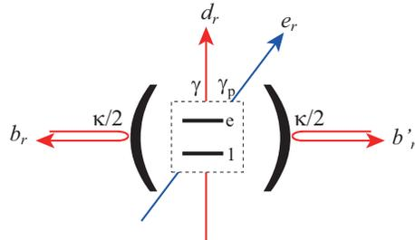
FIG. A1: The cavity-QED setup considered. A matter qubit is confined in a two-sided cavity, and a single photon is input from the left-hand side.
