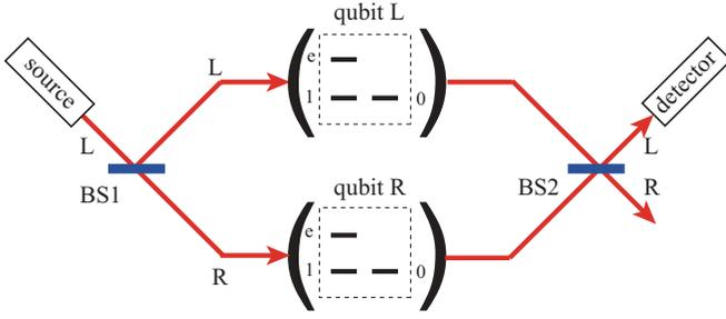
FIG. 1. (Color online) Schematic view of the optical circuit. A single photon is split by a beam splitter (BS1) and is sent to cavities that confine matter qubits with an L-type structure. After interacting with the matter qubits, the photon is combined by another beam splitter (BS2). When the photon reaches the target port and the detector clicks, entanglement is generated between the remote matter qubits.
