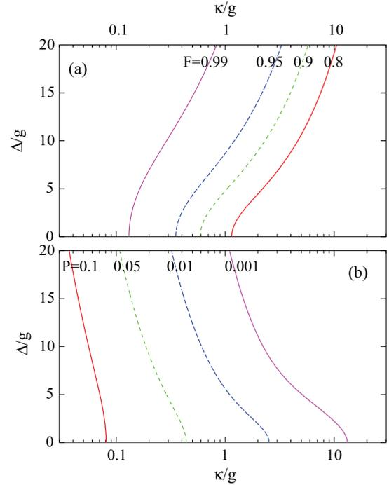
FIG. 3. (Color online) Contour plots of (a) fidelity and (b) success probability as functions of the cavity decay rate  $\kappa$  and the detuning  $\Delta$  in units of the cavity coupling strength  $g$ .  $\gamma_p = \gamma = 2g$ . Even when  $\kappa = 2g$ , high-fidelity operation ( $\mathcal{F} = 0.9$ ) is possible by setting  $\Delta = 9g$ . The success probability will then be  $\mathcal{P} = 0.13\%$ .
