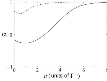
FIG. 3. Dependence of the two-photon Kerr effect  $\alpha$  on the pulse delay  $a$ . The coherence length  $d$  of photons is chosen at  $d = 5.5\Gamma^{-1}$  (solid line) and at  $d = \Gamma^{-1}$  (dashed line).
