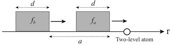
FIG. 2. Profile of rectangular input photons. Both photons have the same pulse length  $d$  and are resonant with the atom.  $a$  denotes the delay of the second photon.
