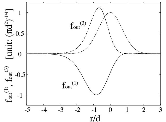
FIG. 2. The forms of the linear (solid curve) and third-order nonlinear (dashed curve) components of the output field. The thin dotted line shows the input field. A moving coordinate system at the light velocity is employed for the horizontal axis. The cavity parameter is  $\kappa/g = 5$  (weak coupling regime), and the parameters for the input pulse are chosen as  $g^2d/\kappa = 1$  and  $q = 0$ . The input and output fields become real after removing the natural phase,  $e^{i\omega_c r}$ .
