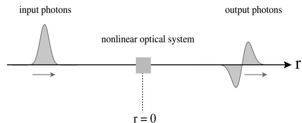
FIG. 1. Illustration of the input and output photons. The input photons interact with a nonlinear optical system placed at  $r = 0$ , and, after the interaction, propagate into the positive direction.
