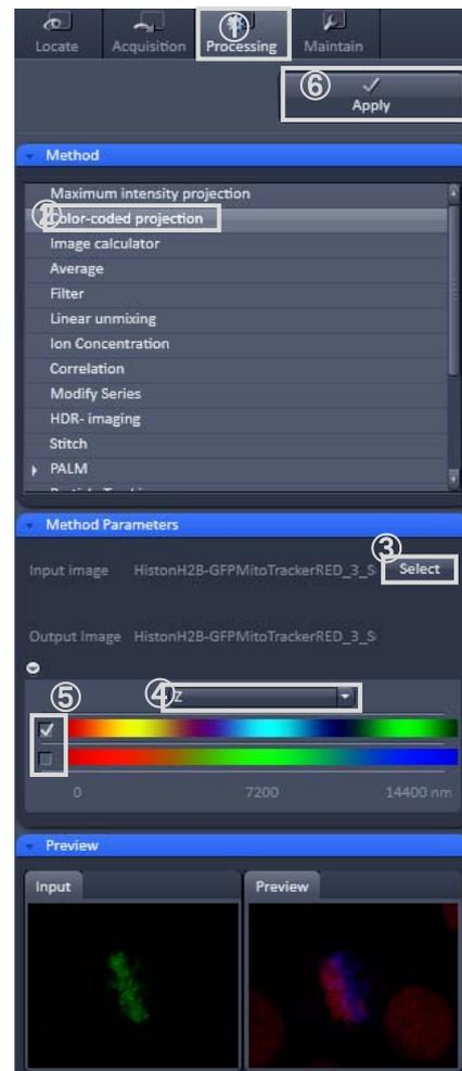
Fig. 60 Color-coded projection
