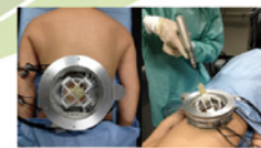
Body-mounted compact surgical robots
