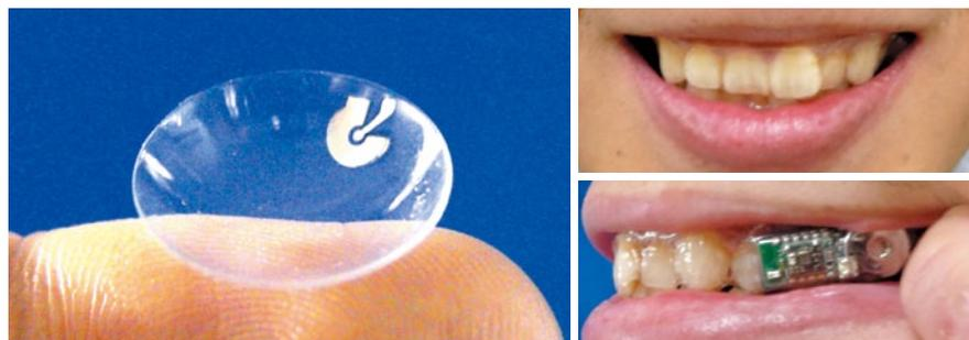
Soft contact lens-type biosensor with biocompatible polymers for tear glucose monitoring (left); Mouthguard telemetric sensor (right: front & side views) with Bluetooth 4.0 LE (low energy) transmitter
