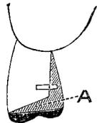
The bar intended to be anchored in the slot cut in the molar on the left side is made of platinum wire, about No. 15 U. S. standard gage, with the end shaped as shown in Figs. 362, 367, and 368. It may be fastened with wax to the artificial tooth and adjusted in the mouth to determine accuracy of position before investing.
