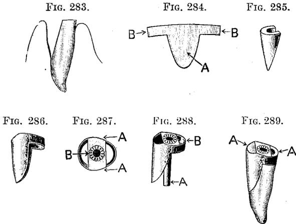
tooth. A piece of round platino-iridium wire which perfectly fits the tube is passed through the tooth and held in position while the tooth is broken away from the tube, thus preventing the marring of the tube, providing a strong platinum tube with a pin which fits it exactly. A suitable tube may be formed out of platinum foil or very thin plate.
