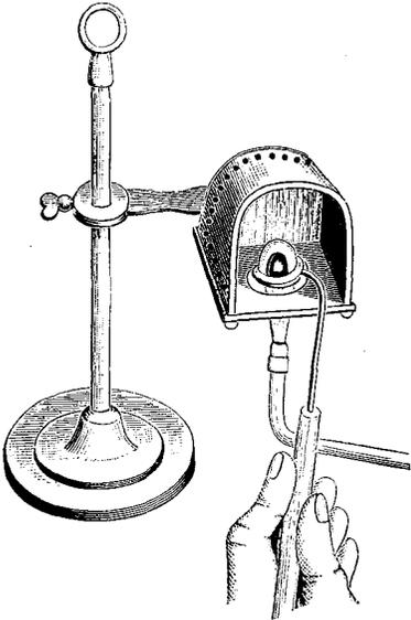
glass drop-tube a little more alcohol. During the packing aid the precipitation of the particles of the body by a few light taps on the side of the fusing-cup or on its handle.
