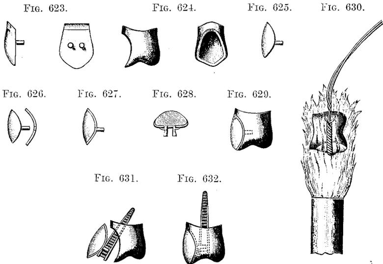
with No. 34 or 36 gage pure gold, punching holes in the backing for pins, annealing as required to readily conform it to the tooth (Figs. 626 and 627). With a sharp knife cut a barb on each side of the pins in the facing, and press the barbs against the backing (Fig. 628), which keeps the backing in place. Burnish down the edges well, being careful not to let the backing overlap the facing.
