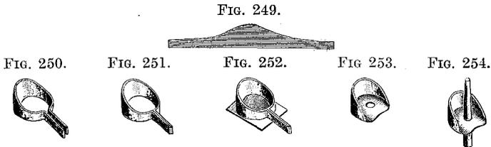
**Post and Disk Method.**—Ready-made posts corresponding in size to the Ottolengui reamers, Fig. 96, with prepared disks of platinum, can be used to facilitate the construction of crowns of this style.
