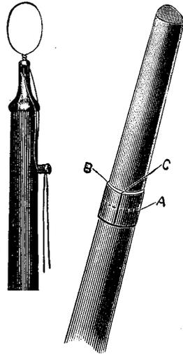
and twist the ends with the pliers until the loop fits tightly at every point (Figs. 130 and 131). Slip off the loop, cut it in the center, and extend the ends lengthwise in opposite directions, as shown in Fig. 132. Then lay it on the surface of the plate of which the collar is to be constructed, and mark the length. Cut the metal beyond this mark sufficiently to allow for an overlap; bevel and lap the ends to the mark and solder them.
