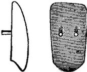
the cap and backing together. The backing must be made thick with solder, the holes in it deepened with a drill, and the pins of the porcelain front serrated and fitted therein. After the final soldering, the porcelain fronts are cemented in position with oxyphosphate. This method, though affording sufficient attachment for a short molar, such as is illustrated in Fig. 465, is suggestive of insecurity for most of the front teeth.
