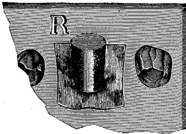
After a minute or two the mold may be reversed, the hubs shaken out, and the casting process continued until a considerable number of hubs shall have been made. In Fig. 201 a molar hub is shown in place on a piece of No. 32 gold plate, which lies over the upper right first molar die. A succession of blows on the hub with a four-pound smooth-faced hammer will drive the
