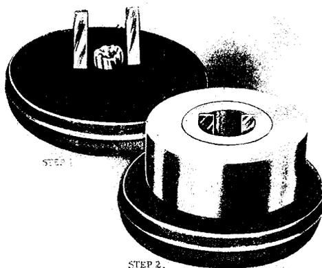
a flask of this kind, "the Turner." The form of the tooth to be molded is placed in the center, occluding surface up. The molding ring is set around the tooth form (small diameter up) and
