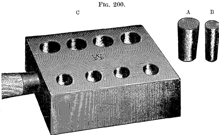
four parts, melted together. The mold C should be warmed, the metal alloy poured in every hole, and the overflow wiped off just before the metal stiffens;
