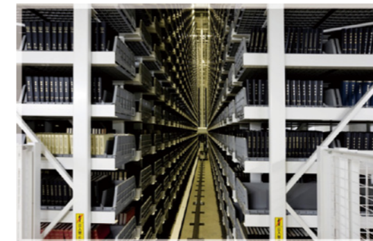
自動書庫 (M&DタワーB1, 2F) Automated Storage and Retrieval System (M&D Tower, B1, 2)
